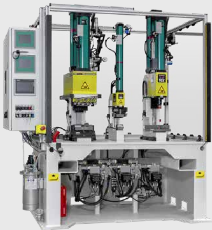
TOX®-Press for eClinching of fuse parts.
